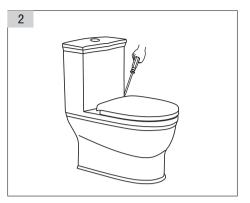
2. Install the cover to the toilet according to the cover installation manual.
